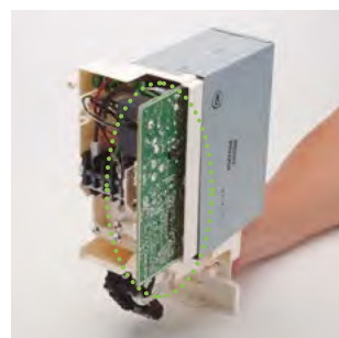
Simple steps for PCB removal.
